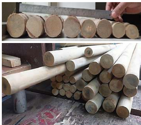
D. stocksii in different dimensions and smoothened standard round rods.
