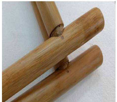
Bamboo component after coating with melamine.
